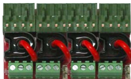
SL-SENSOR2 / SL-SENSOR4 3 Wire Speaker Line Short Sensor
