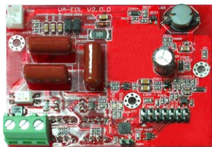
VA-EOL End of SP-line Module for Multi-branch/3-wire
