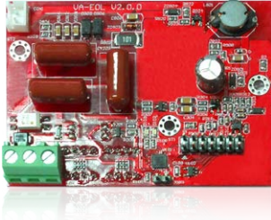
VA-EOL End of SP-line Module for Multi-branch/3-wire
